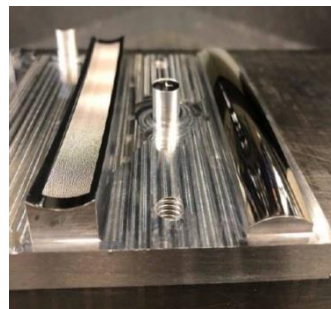
Non-Planar Patterning by CNC Machining
