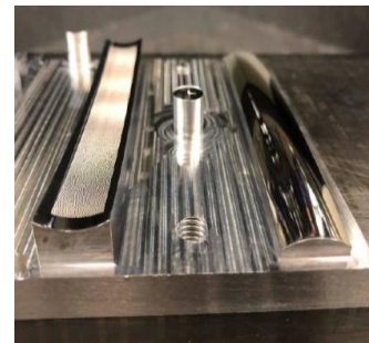
■ Non-Planar Patterning by CNC Machining
